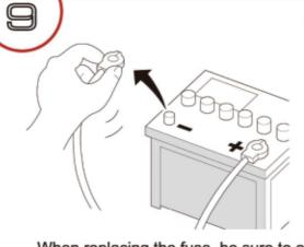
To avoid potential shorts in the electrical system, be sure to disconnect the (-) battery cable before installation. Use this unit with a 12-Volt battery and negative grounding only. Failure to do so may result in a fire or malfunction.
